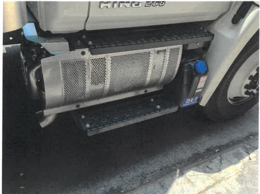
Hino truck and its selective catalytic reduction (SCR) next to the Diesel particulate filter (DPF) with regeneration process by the late fuel injection to control exhaust temperature to burn off soot. (Courtesy of: Wikipedia)
